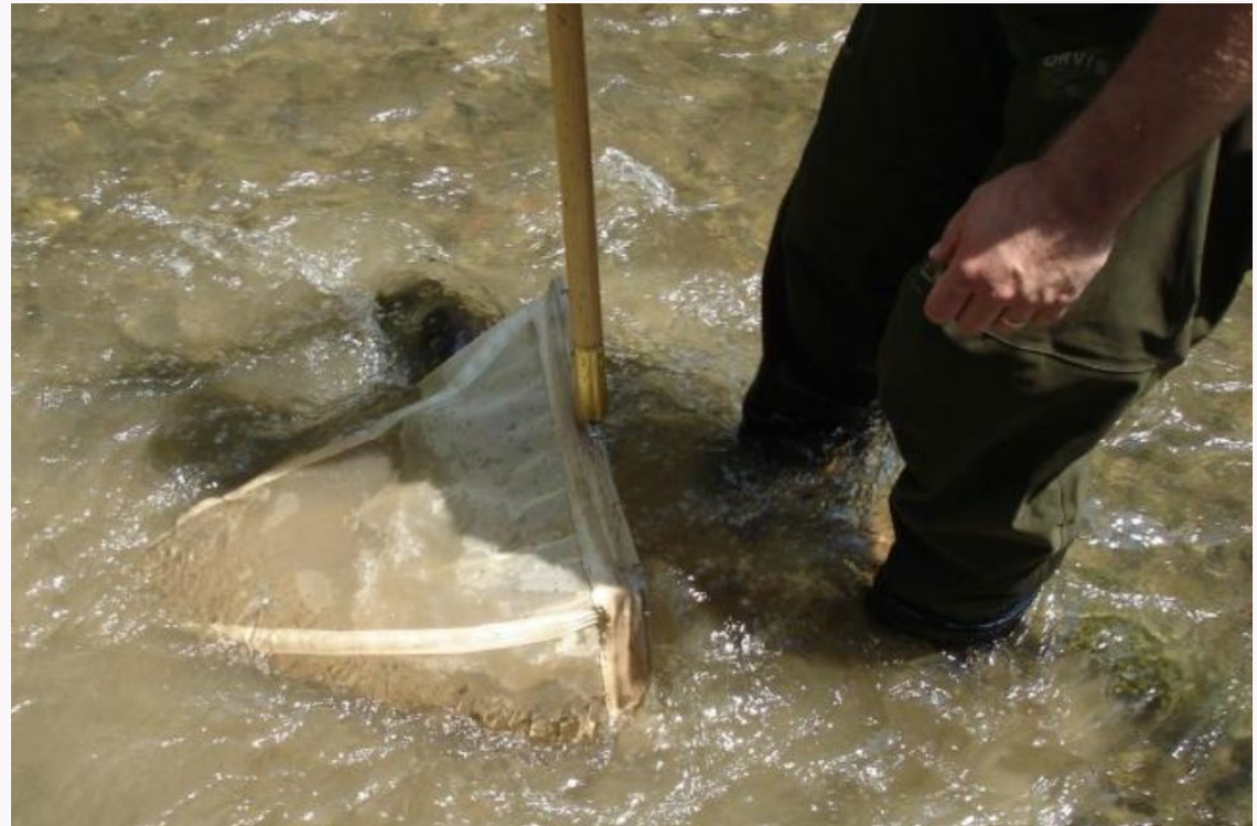
D-net sampling method for macroinvertebrates
